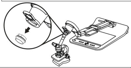
If the eyepiece is Ø 28 mm or Ø 31 mm, you need two microscope adapters. (1. The Lumens microscope adapter. 2. The microscope adapter suitable for the eyepiece size Ø 28 mm or Ø 31 mm).
